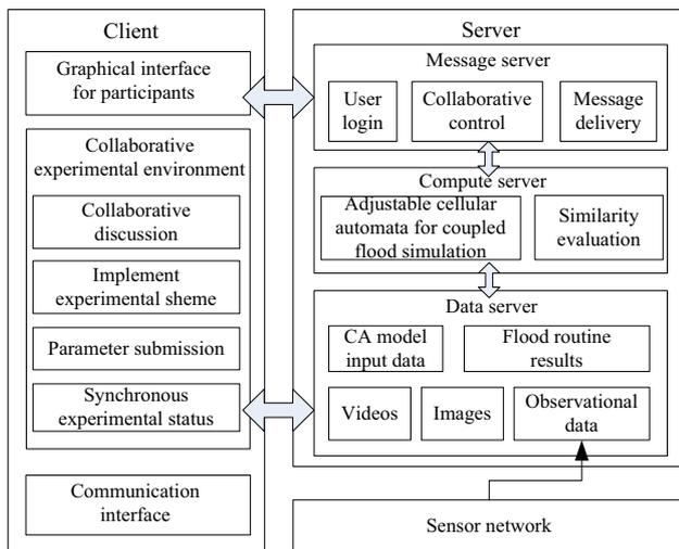
**Fig. 3** Construction of a collaborative flood experiment environment system
