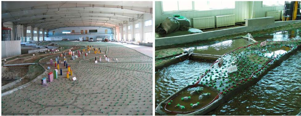
**Fig. 4** The physical model of the Hunhe River
